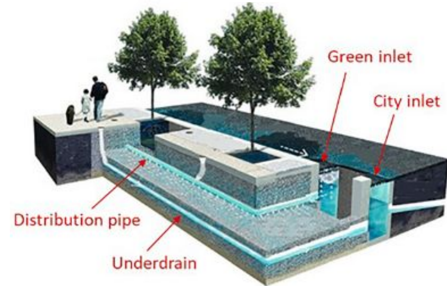
Stone trench with embedded tree pits (i.e., tree trench) underneath a sidewalk on North 7th Street in Philadelphia, PA
