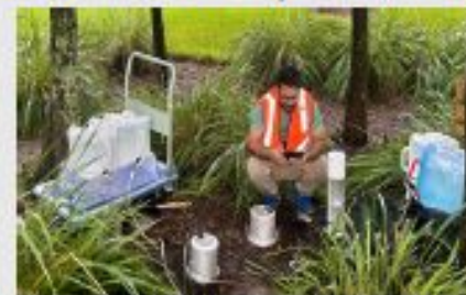
Measurements of soil hydraulic characteristics in the rain garden
