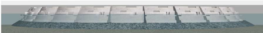
Living Shoreline in-situ elevation looking west. Conceptual drawing shown without plants. Approximate scale 1/8"=1'.
