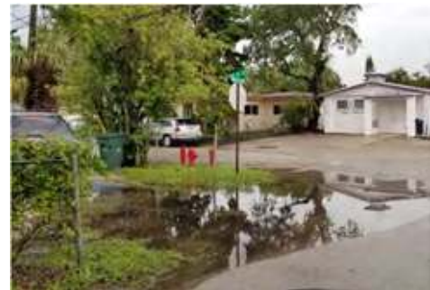
NW 8 th Court/NW 17 th Avenue – June 6, 2017. Example of isolated low area without inlet(s) for collection.
